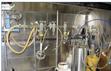
Gas transfer manifold
